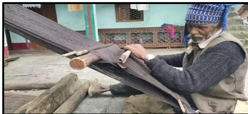
Fig.-7: Other End Of Taana Attached With The Belt Around The Weaver
