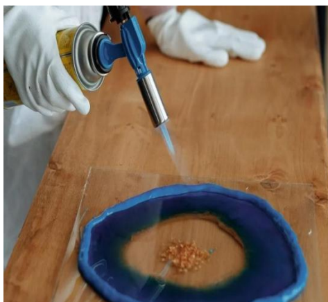
Fig-9: Removing Air Bubbles using Heat Source
